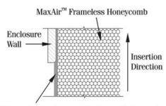
Soft, conductive foam perimeter gasket grounds the honeycomb directly to the enclosure.
